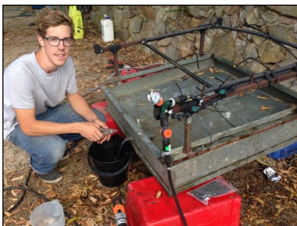
Calibrating the rainfall simulator
